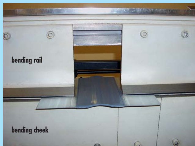
A bending machine with removable rail parts. © Semmler GmbH 2011
