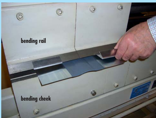
A bending machine with a metal shoe. © Semmler GmbH 2011
